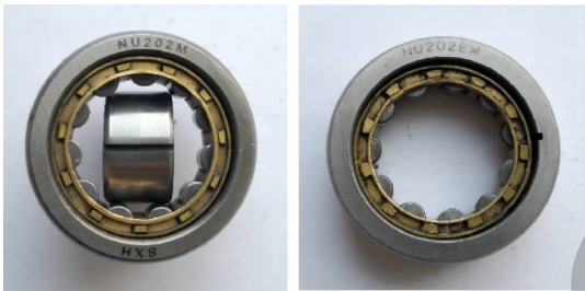
图 5 带局部故障的中介轴承 Fig. 5 Inter-shaft bearing with local failure
